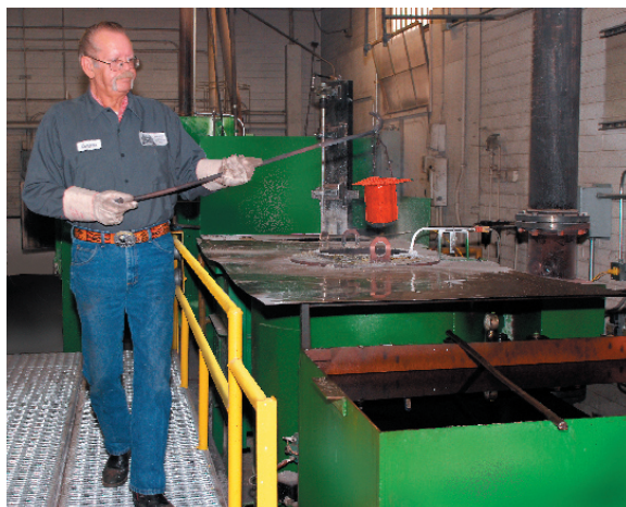
PHT ramped up the salt line to support a higher volume of tool steel hardening with overnight delivery. Lab results showed that improved heating rate uniformity reduced cycle times, improved quality and product yield. Most common tool steels are now processed in one cycle with greater efficiency at a lower cost, and without sacrificing quality.
