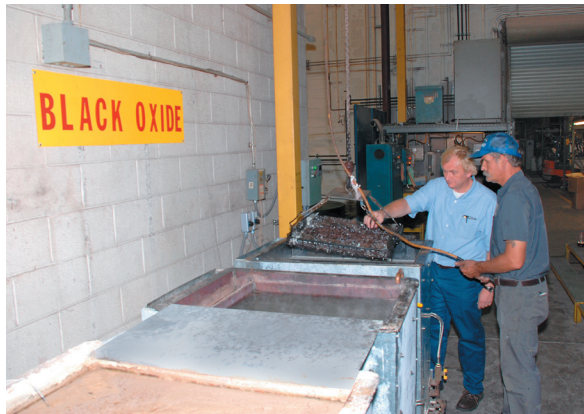
PHT's black oxide can be produced at lower temperatures and the metal finishing process produces a low cost, protective surface that is corrosion protected and abrasion resistant.
