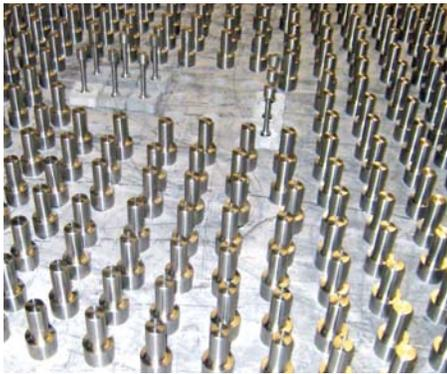
**Figure 4.** PH steel explosion bolts were stress relieved in +/- F uniformity and re-solution treated in a uniform manner to achieve the required mechanical properties. The spacing of the bolts on the heat treating rack is well-defined.
