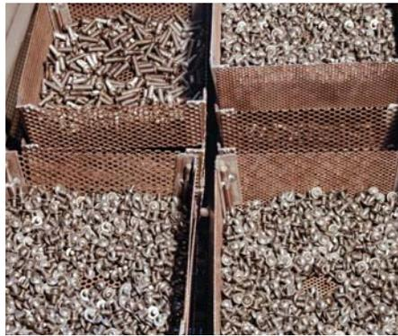
**Figure 5.** Example of stacked baskets containing 4037 cold-head cap screws for heat treating. Notice the screws are spread out and stacked in layers to reduce density and improve response to quench.
