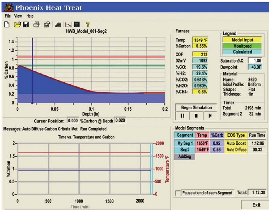
**Figure 1.** Super Systems, Inc. CarbCALC software used on carburize and carbonitriding cycles. The process cycles can be customized to meet the material chemistry of your parts. Verification of every step in the processing cycle is time-stamped and recorded.
